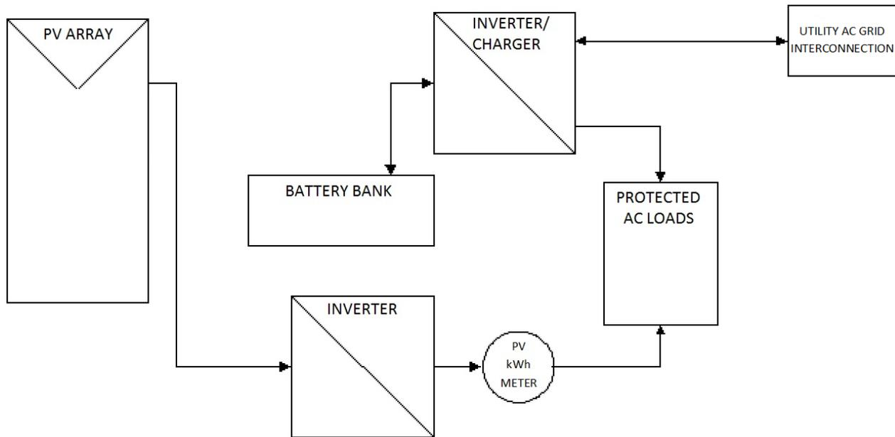
Figure 5. AC coupled multimode system
