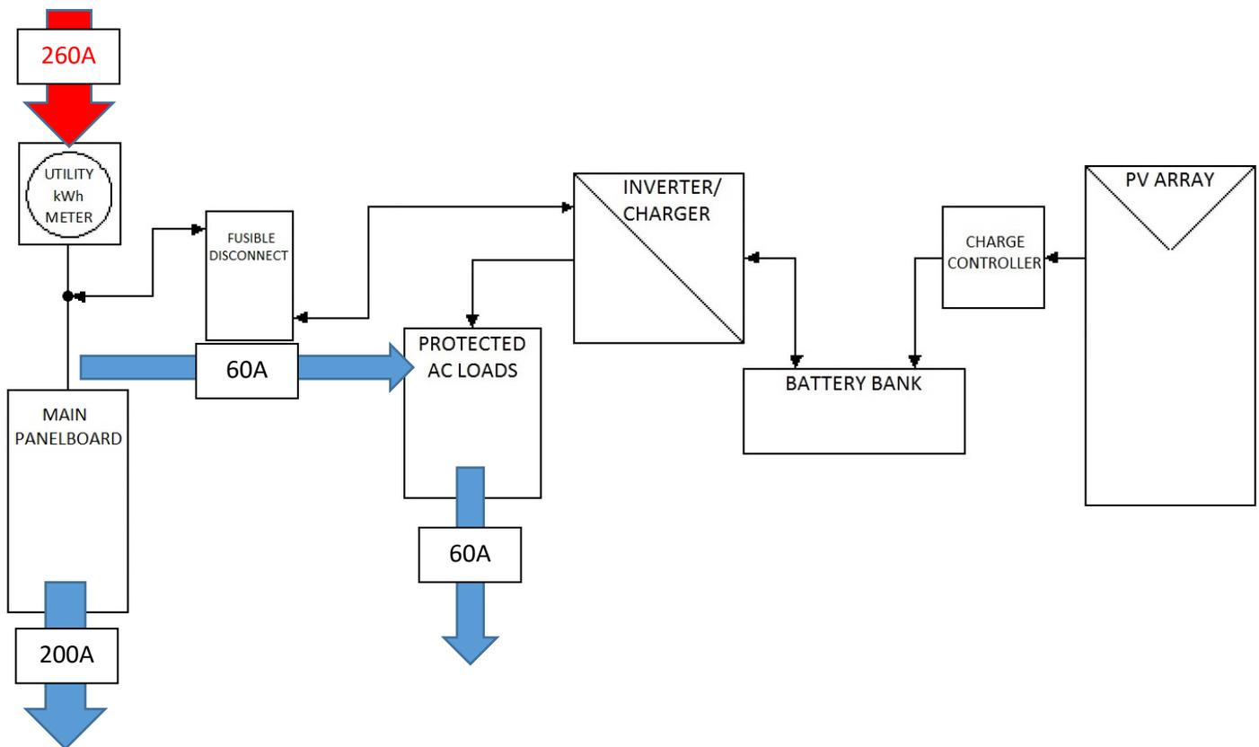
*Figure 8. Example of supply-side connection with overloaded service conductors*
