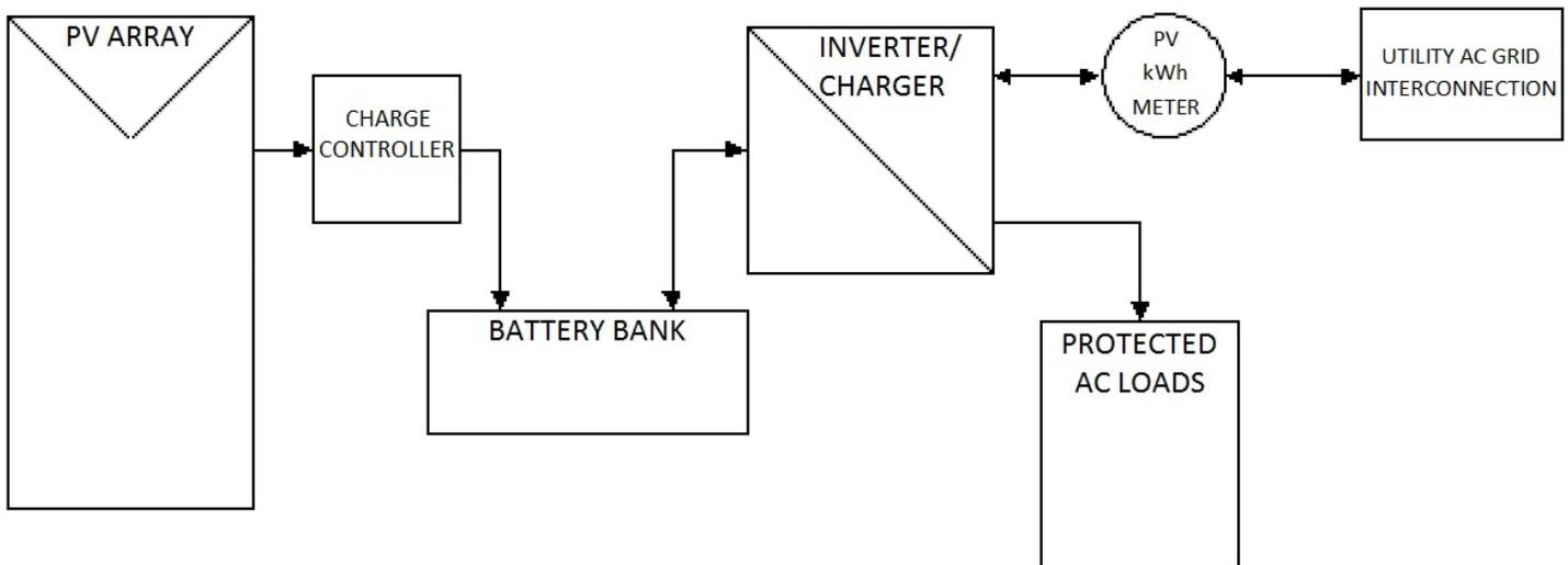
Figure 4. DC coupled multimode system
