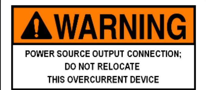
Figure 11. Example of “do not relocate” label for backfed overcurrent device when Article 705.12(B)(2)(3)(b) is utilized
