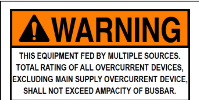
Figure 12. Example of label required for “AC combiners” indicating multiple sources, and not to add loads
