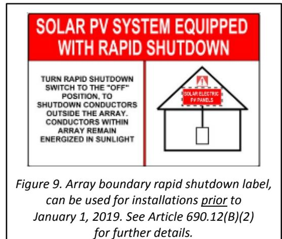
Figure 9. Array boundary rapid shutdown label, can be used for installations prior to January 1, 2019. See Article 690.12(B)(2) for further details.
