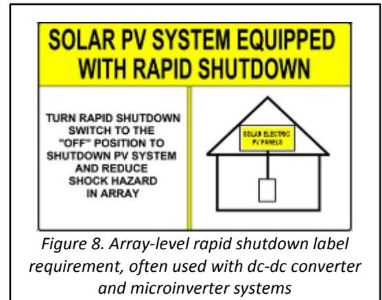
Figure 8. Array-level rapid shutdown label requirement, often used with dc-dc converter and microinverter systems
